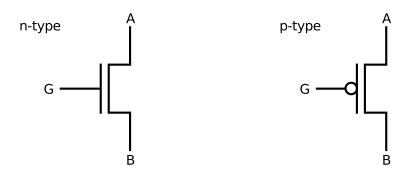
The nMOS and pMOS transistors differ in how they switch based on the input G (called the Gate).
